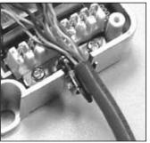
3. Place the end of the cable jacket onto the cable clamp so that the wire pairs can easily be positioned as needed inside the Box.
