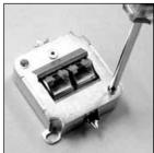
Unscrew and remove the cover plate (above left) from the Box, then unscrew and remove the inner cover (above right) to reveal the color-coded pins inside the unit.
