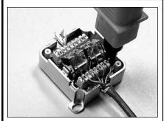
Use a Krone punch-down tool to crimp each pair of wires and connect them to their corresponding color-coded pins.
