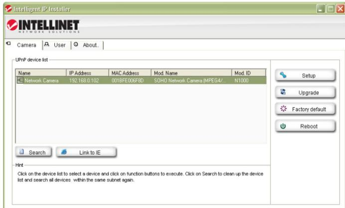
When the program starts, you are presented with the screen shown above. The IP Installer utility lists all cameras that can be found on your network. With this utility you can make changes to the configuration, perform a firmware upgrade, restore the camera to factory default values, and reboot the camera. Note: It may take up to three minutes for IP Installer to show a camera that has been recently (re-)started. Refer to the user manual for more detailed instructions on the camera setup.
