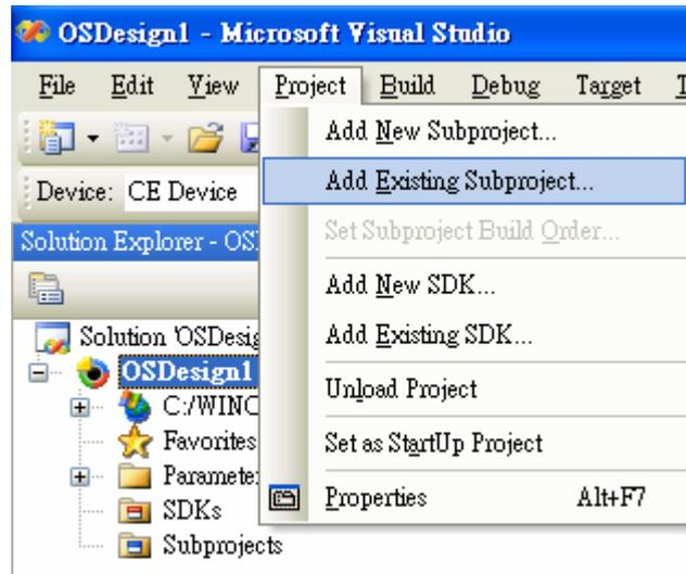
**Step 6:** After the subproject is added, you may configure the “mxupce6.reg” registry file with the location [HKEY\_LOCAL\_MACHINE\Drivers\USB\ClientDrivers\MXU\_11x0].
