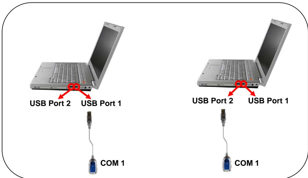
When "Fixed-base COM Mode" is enabled for the first time, all the COM port numbers and serial port parameters will reset to their default values. You can then set the COM numbers and configuration parameters to the values needed for your application(s). Note: If you subsequently disable "Fixed-base COM Mode," all the parameters will be restored to their original settings.
